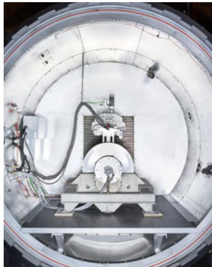
RISING TO THE CHALLENGE The company's levitation rig in Los Angeles uses a vacuum and rotating magnets to test the technology.
